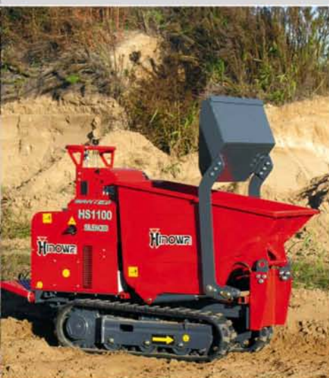
KIT CASSONE AUTOCARICANTE SELF-LOADING DUMPER BED
